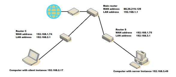
The previous configuration (see *LAN configuration*) does not work in this network scenario because server and client are behind a NAT.
