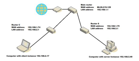
• On the server side, the *WAN IP* field contains the server's router IP address, i.e. the Router S IP address (192. 168.1.75) since Router S NAT settings relay inbound traffic to server's TCP port towards Server computer.
