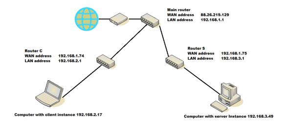
• On the server side, the *WAN IP* field contains the server's router IP address, i.e. the Router S IP address (192. 168.1.75) since Router S NAT settings relay inbound traffic to server's TCP port towards Server computer.
