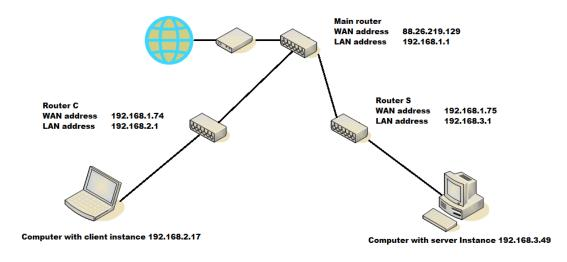
• On the server side, the *WAN IP* field contains the server's router IP address, i.e. the Router S IP address (192. 168.1.75) since Router S NAT settings relay inbound traffic to server's TCP port towards Server computer.
